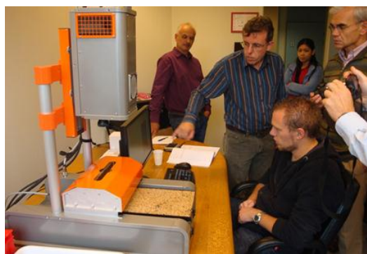
Demonstration of NIR hyperspectral method to determine ergot in grains at an industrial setting
