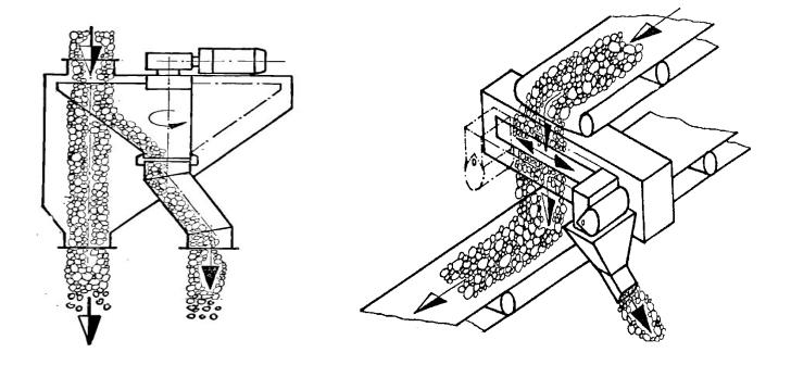
Slit size min 3 x max particle size - the speed the slit should pas depends on the speed of the stream
